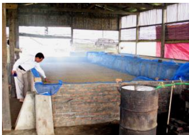
A flat-bed dryer with a 4-ton capacity (Myanmar)
