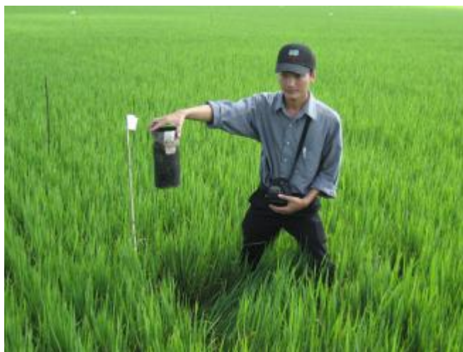
The field water tube is a simple tool used in implementing AWD for deciding when to irrigate fields (Mekong Delta, Vietnam)
